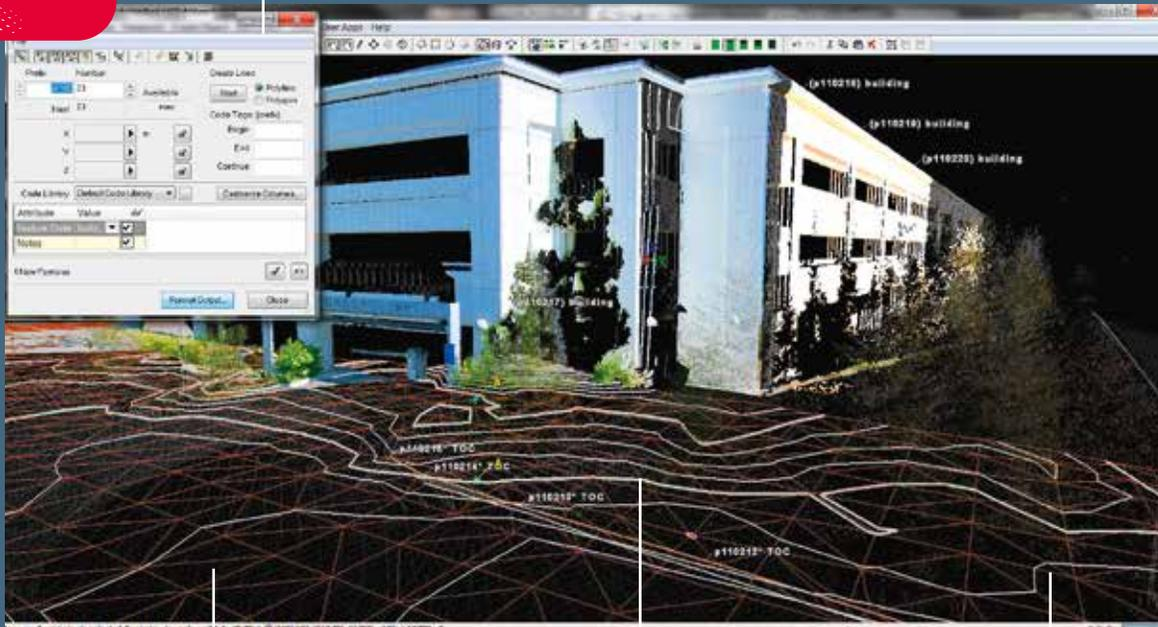
Automatic TIN mesh at any grid spacing
