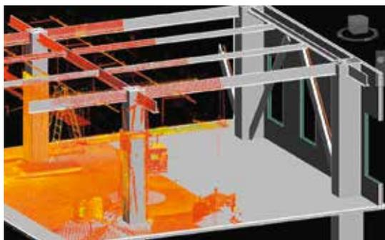
Revit model objects (walls, floors, columns, etc.) can be best-fit to the point clouds which provide accurate as built models.
