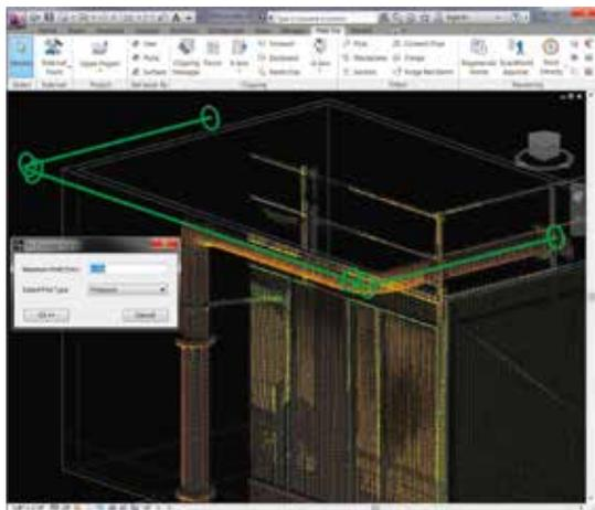
Intelligent point fitting tools assist in finding pipe centerlines and diameters. This ensures users can identify exact and accurate tie points and clashing, a very important part of modeling as-built piping.
