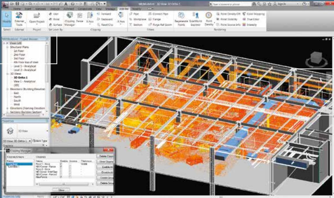
Users can create Revit modeled objects from the point cloud.
